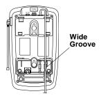
5. Insert the supplied AC adapter's barrel plug into the **DC IN 9V** jack on the back of the base.
